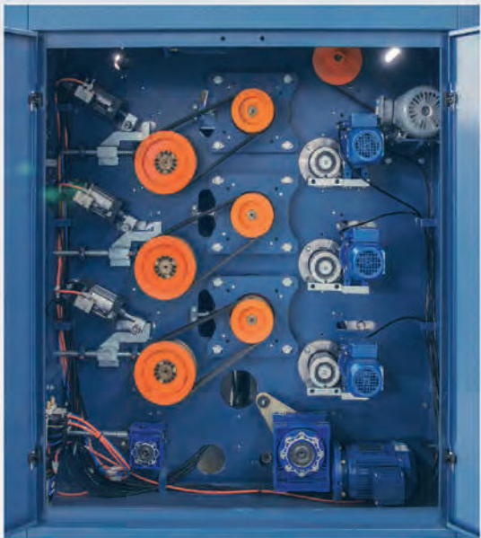
横动装置：每根磨毛辊可独立控制、窜动，可消除织物布面的竖条。 Transverse device :each sueding roller can independent control and moving ,to avoid surface crease.
