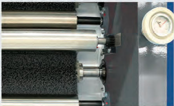
碳丝辊、陶瓷辊、砂布辊可任意互换 Freely combine of carbon fibre roller , ceramic roller and emerying roller.
