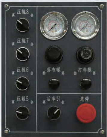
出布侧操作面板，利于出布端压辊调整 Control panel at the side of fabric-out , easy to adjust pressure roller at fabric-out.
